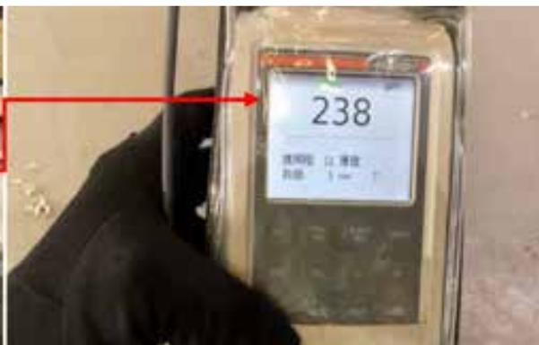
圖 16 鋼構橋梁鍍鋅膜厚度測 ( $1\mu\text{m} = 7.2\text{g}/\text{m}^2$ )
